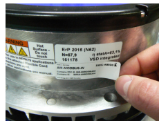
Example: Sticking the "FCC/IC" label "AM-MODBUS-W" onto a fan housing.
